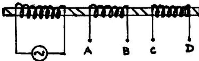
(a) coils AB and CD are in series in the first case while they are in parallel in the second case.
