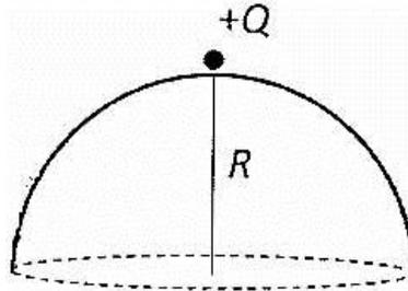
(A) The electric flux passing through the curved surface of the hemisphere is  $-\frac{Q}{2\epsilon_0} \left(1 - \frac{1}{\sqrt{2}}\right)$ .
