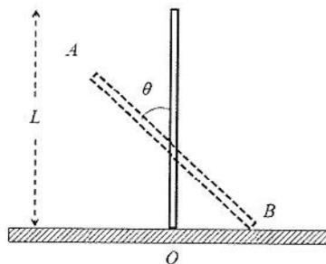
(A) Instantaneous torque about the point in contact with the floor is proportional to  $\sin \theta$
